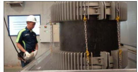
Hydro pressure test-1200mm
