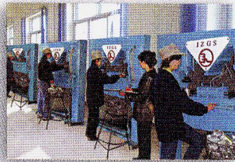
Gas Leakage Inspection
